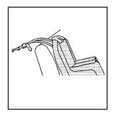
If the position you are using does not have a head restraint and you are using a dual tether, route the tether over the seatback.
